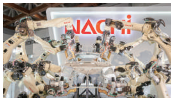
Full-sized robots: The SRA (Used in the machining of EV bodies, etc.)
