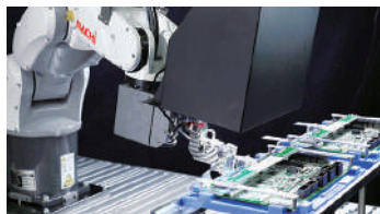
Robot connector insertion applications (to enable automated/high-speed insertion of cables for applications such as smartphones and tablets)
