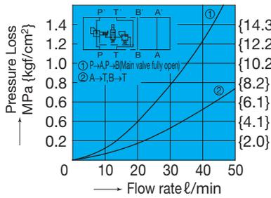
Pressure – Flow Rate Characteristics
