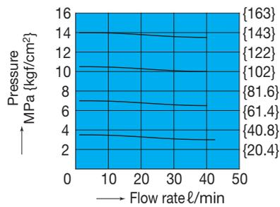
Pressure – Drain Rate Characteristics
