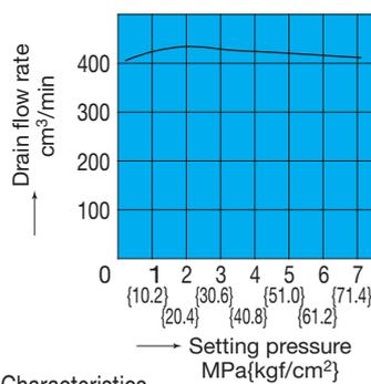
Pressure – Drain Rate Characteristics
