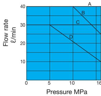
Note) 1. The maximum flow rate is the value when a rated 90%V is applied following solenoid temperature rise and saturation.
