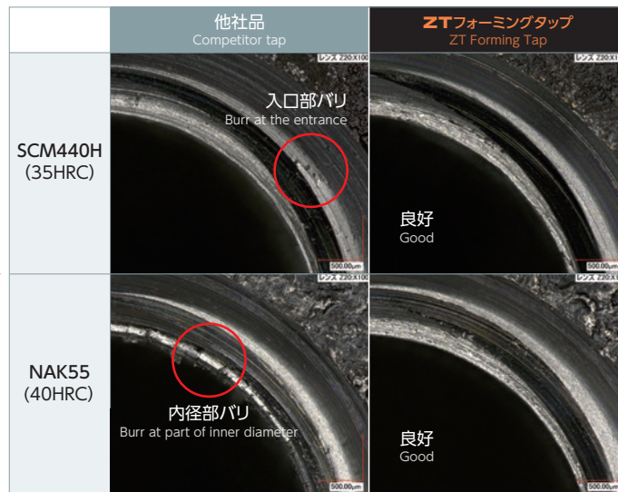
めねじのバリ比較 Comparison of internal threads burr
